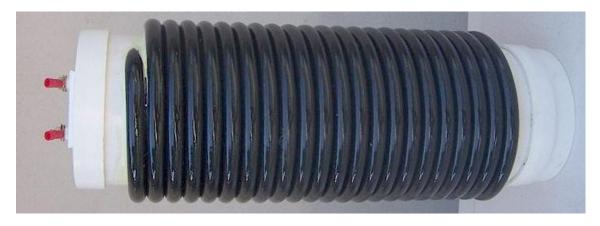
Each end can be terminated in the coax connector of your choice or one end can be terminated in terminals (nuts and bolts perhaps) for connection of a balanced line.
