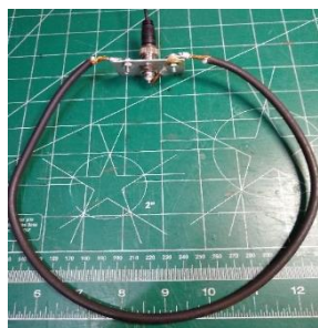
Figure 12 Driven loop connections to feedline
