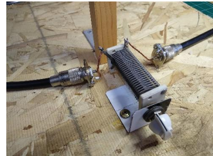
Figure 7 Breadboarded capacitor for first contact
