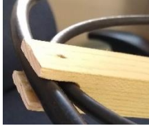
Figure 13 Notch at top of mast for loops
