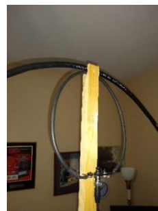
Figure 3 How the driven loop is positioned
