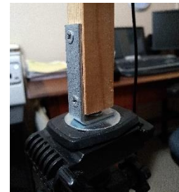
Figure 16 L-bracket for mounting to the tripod
