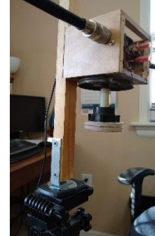
Figure 14 Capacitor Box Assembly mounted six inches from the bottom of the mast
