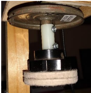
Figure 15 Nylon coupling and knob assembly
