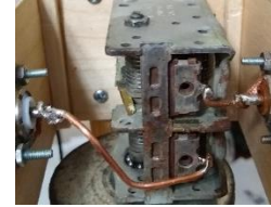
Figure 10 Capacitor Sections Connected in Series
